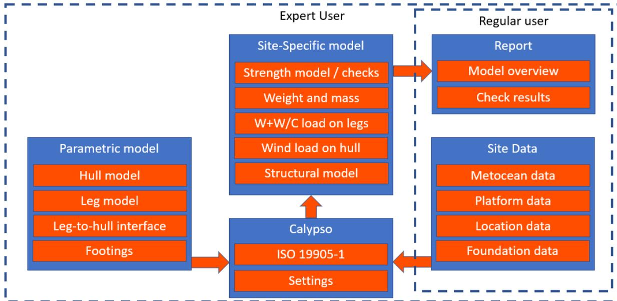
**Figure 2 : Schematic overview of Calypso**
